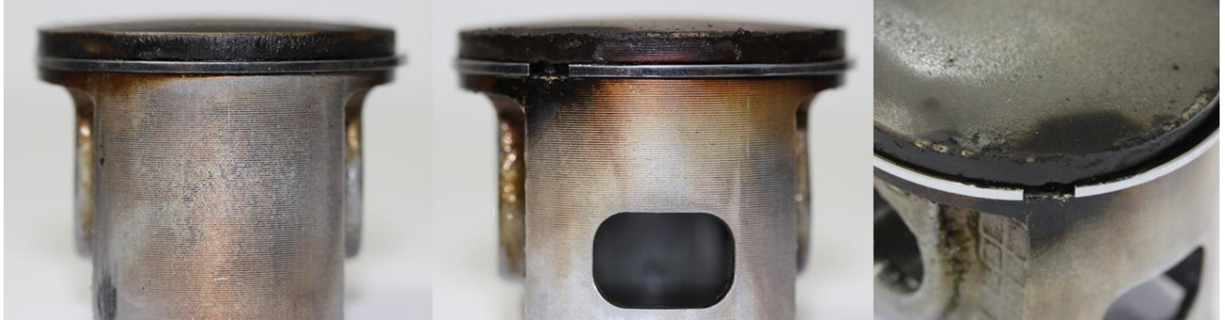
Figure 9: Piston views (150.4 hours + previous ~30 hours)
