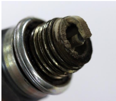
Figure 14: Spark Plug (150.4 hours)
